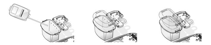
31. The cassettes are placed in the ice container in the LifePort<sup>™</sup> by the SRC. The tube frame must be perpendicular to the pump deck and the hinges must be positioned inside of the receivers on the pump deck. Keeping the hinges in place, turn the tube frame down flat onto the pump deck.
