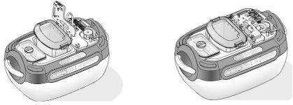
32. The SRC opens the pump head and stretches the tubing over the wheel. The SRC closes and latches the pump head raceway to clamp the tubing. She/he rotates the pump deck locking arm 90° and snaps into place. She/he connects the pressure sensor cable from the pump deck to the connector on the tube frame. She/he presses the POWER button on the control panel to energize the unit. The SRC checks the outer display and verifies that the top line reads "Ready". See the Illustration 4 below.
