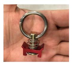
\*Note: Fasteners (pictured above) are provided by aircraft to secure OCS<sup>™</sup> HEART Machine and should be set up in a similar fashion as seen in Gulfstream Astra SPX (Configuration A pg. 15-17).
