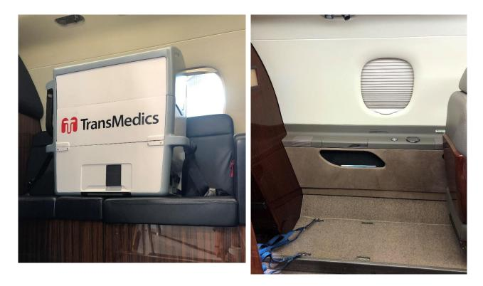
\*Please note that the OCS<sup>™</sup> HEART Machine may be secured on the extra seating (see left above) or to the floor (see right) if the seat is removed and should be secured to the grips on the aircraft floor.
